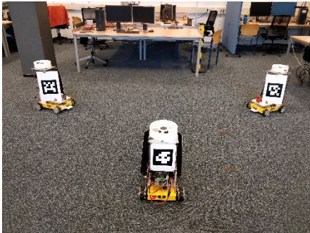
Monocular camera with tag recognition [1]
